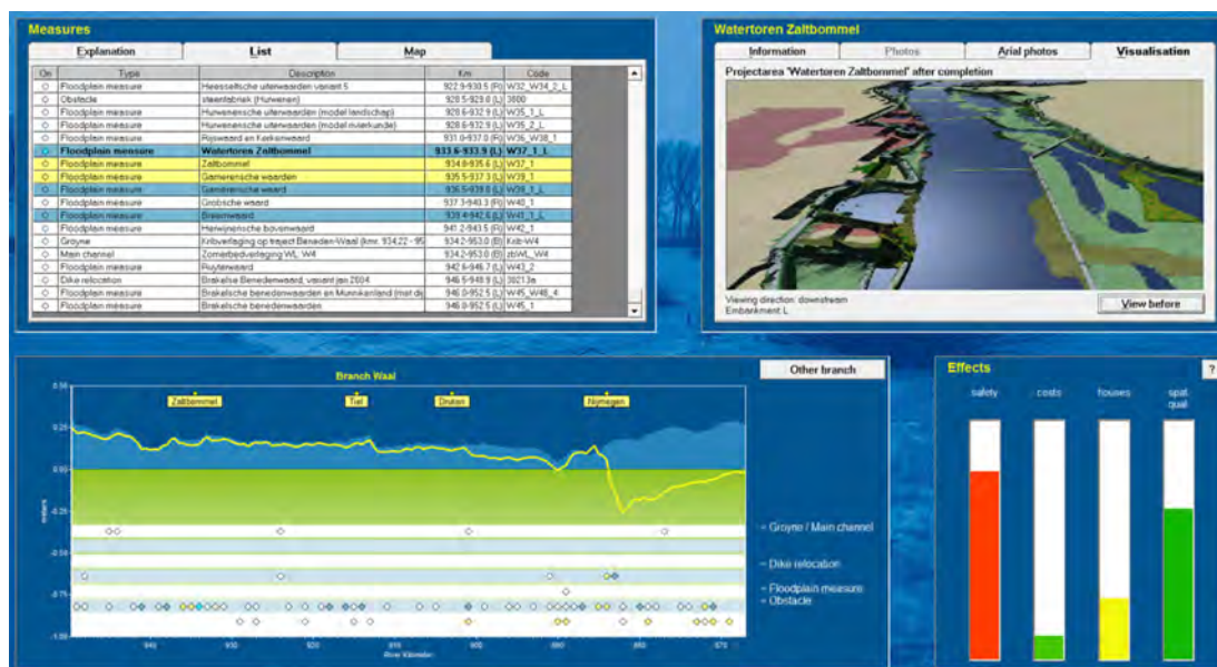
Figure 16 — Example of planning kit dashboard for Room for the River project, showing measures, reduction of design flood levels and other impacts (Deltares)
