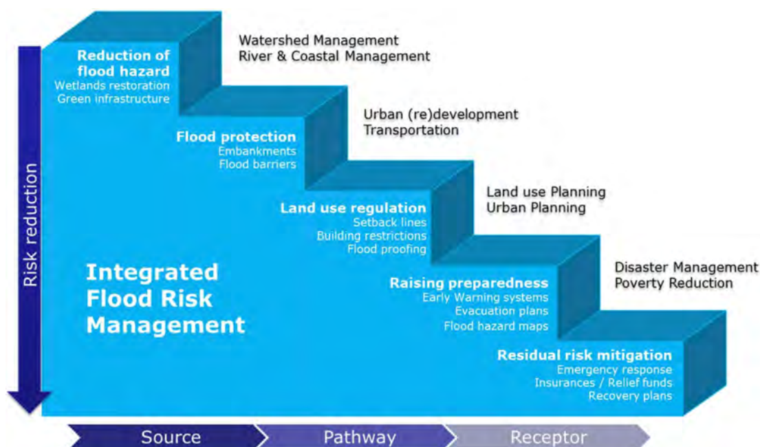
Figure 4 — Cascade with potential integrated flood management measures and associated policy and management fields (adapted from Marchand et al., 2012)
