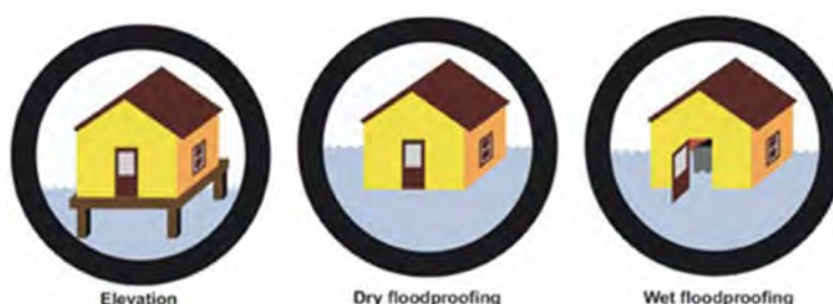
Figure 12 — Different methods of floodproofing (adapted from FEMA, 1986)
