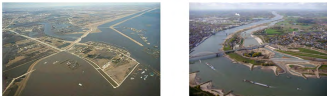
Figure 7 — Enhancing flow conveyance: Red River Floodway at Winnipeg, Canada (left) and side-channel of Waal River at Lent, Netherlands (right) (Manitoba Floodway Authority, Canada, left; Ministry of Infrastructure and Environment, Netherlands, right)
