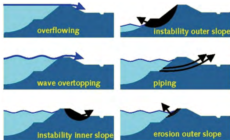
Figure 8 — Failure mechanisms of an embankment (Netherlands Ministry of Infrastructure and Environment)
