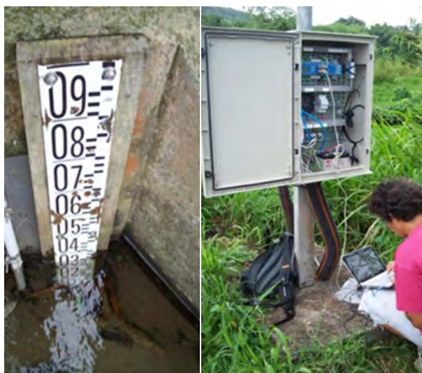
Figure 17 — Hydrological monitoring: staff gauge (left) and data-collection platform (right) (Paul Pilon)
